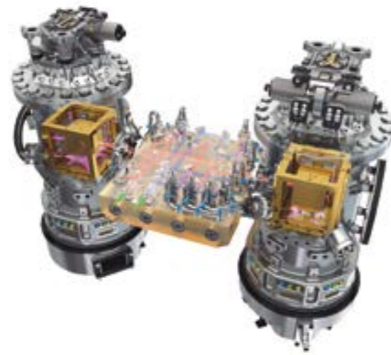
Figure 15: ESA's LISA Pathfinder payload, the "LISA Technology Package" (LTP), where all of the mission's science experiments were performed. Credit: ESA.
