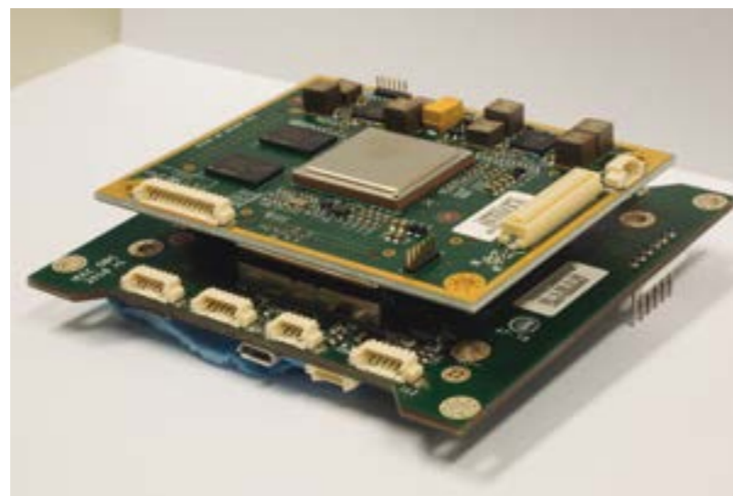
Figure 3: Image of the C3SatP Flight Model with an OBC (On Board Computer), an OBDH (On Board Data Handler, for high-performance calculations and operations) and an SDR (Software Defined Radio, dedicated to communications). Credit: IEEC.
