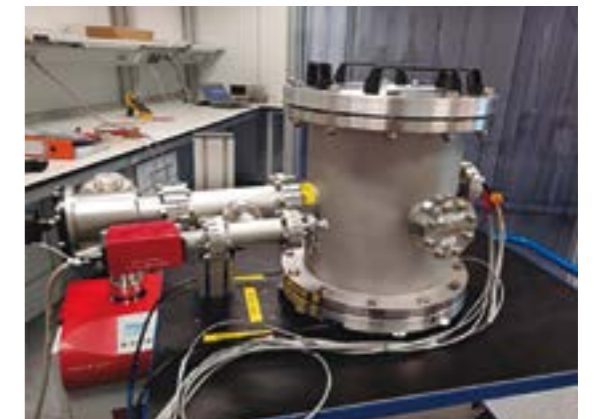
Figure 17: LETS test bench. The vacuum chamber includes a series of active and passive thermal shields to isolate the sensors inside from external temperature fluctuations.
