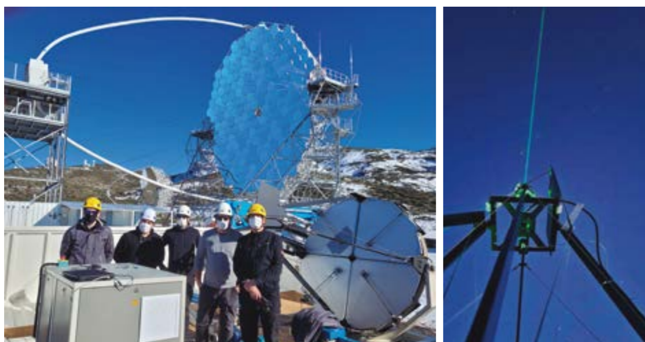
Figure 12: The Barcelona Raman LIDAR after installation, seen in front of the LST-1 telescope (left); the green part of the laser beam can be observed, after exiting the system (right). Credit: Paolo Calisse (CTAO).
