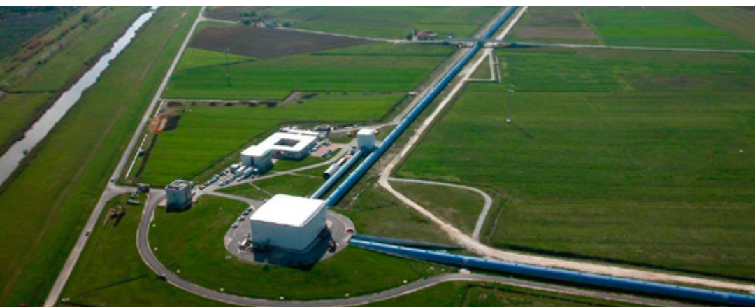
Figure 44: Aerial view of the Virgo site showing the Mode-Cleaner building, the Central building, the 3km-long west arm and the beginning of the north arm. Credit: The Virgo collaboration/CCO 1.0
