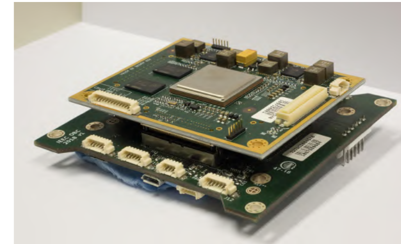
Figure 10: Image of the OBDH and OBC boards of the Catalan Cubesat Platform developed at IEEC.
