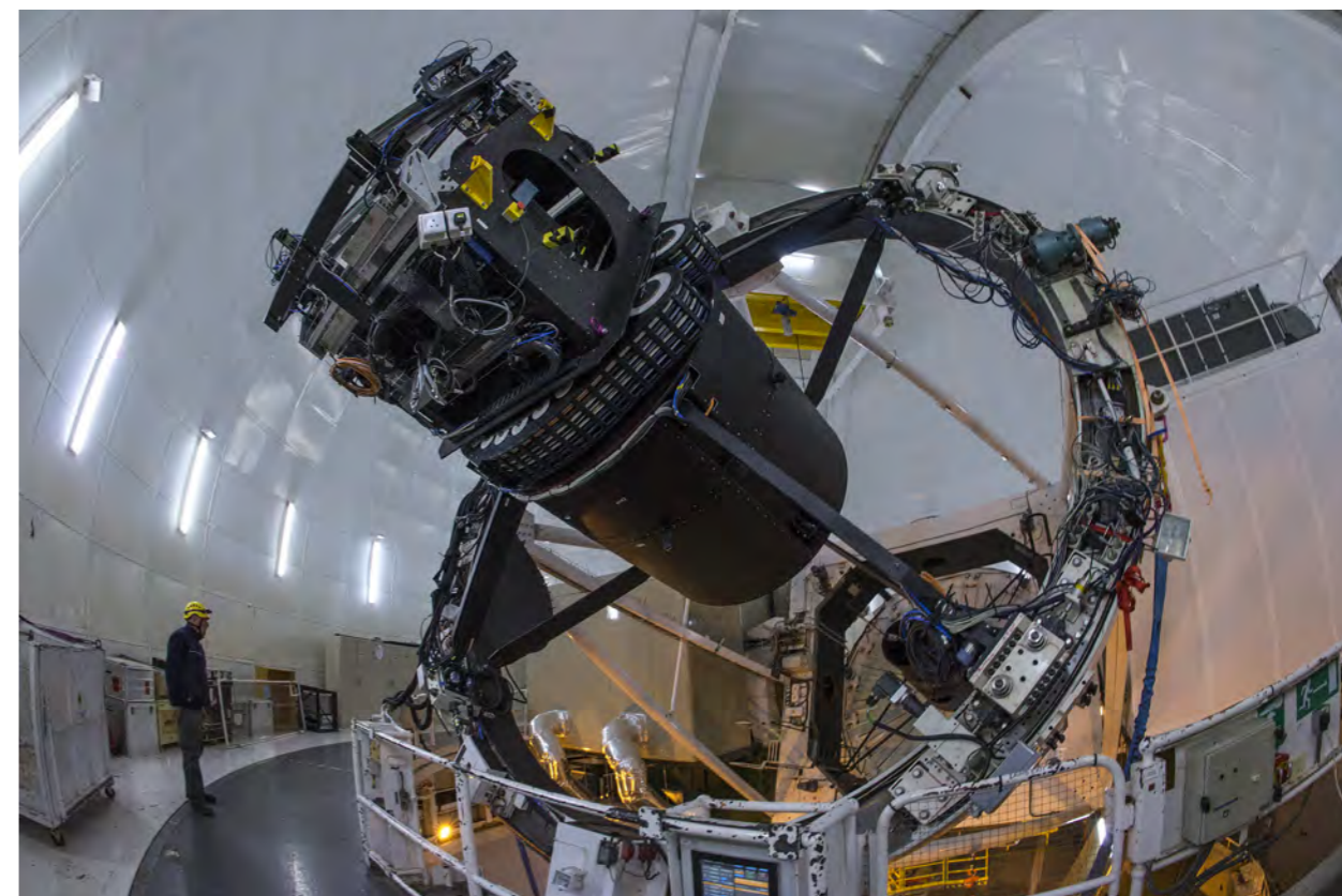
Figure 20: The WEAVE instrument mounted at the top ring of the William Herschel Telescope. The fibre positioner system is located at the black box, and fibres transfer light into the Nashmidt platform at the side of the telescope. Credit: Javier Méndez.
